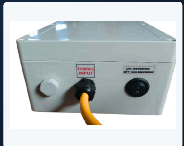
Waterproof switch and ventilation design
